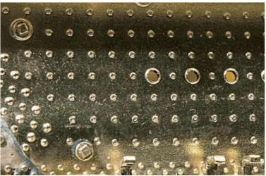
The washout plugs are soldered in place using small individual castings as are the blowoff cocks. The full detail extends around the front lower face of the firebox as it should while this area does not exist on the Samhongsa model. All Kohs & Company models have been modeled in this fashion.
